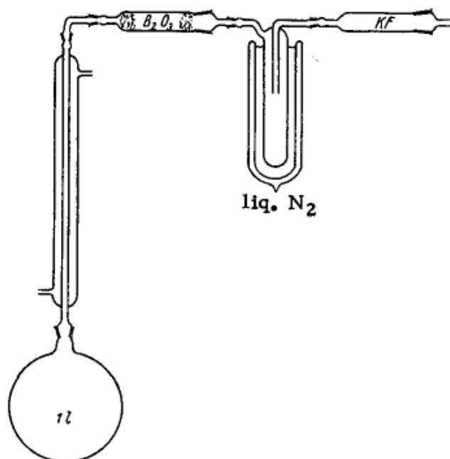
Fig. 133. Preparation of boron trifluoride.
