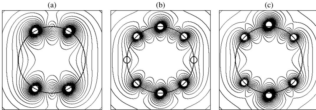
**Fig. 3.** Contour diagrams of the magnetic field in the coil midsection: (a) saddle coil; (b) birdcage resonator; and (c) our coil. The lines are drawn with a step of 0.05; the field at the center is assumed to be 1.
