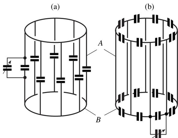
**Fig. 1.** (a) Lowpass and (b) highpass modifications of the birdcage resonator.
