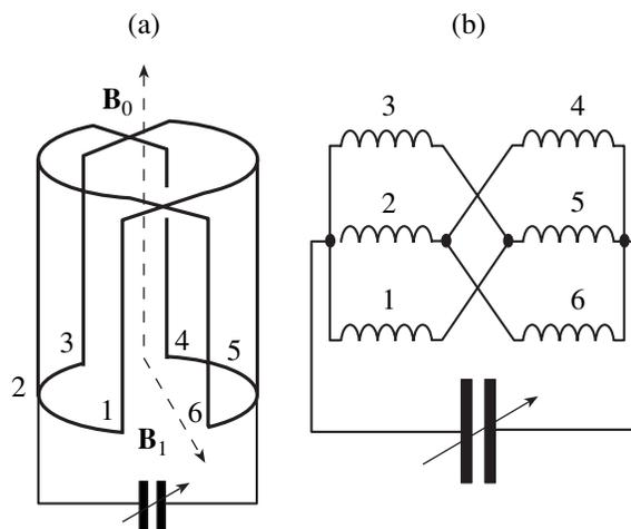
**Fig. 2.** (a) 3D presentation and (b) circuit diagram of an NMR probe coil.
