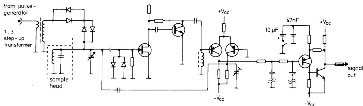
Fig. 2. Basic circuit of the Robinson oscillator. As a variation of Robinson's original circuit, a pair of diodes couples the pulse generator to the sample circuit. Another pair prevents the amplifier input from going into saturation as a result of the large high-frequency pulse applied. The two  $\pi$ -filter capacitors can be disconnected to reduce the recovery time. A detailed description of the complete circuit can be found in Robinson's paper (Ref. 12).
