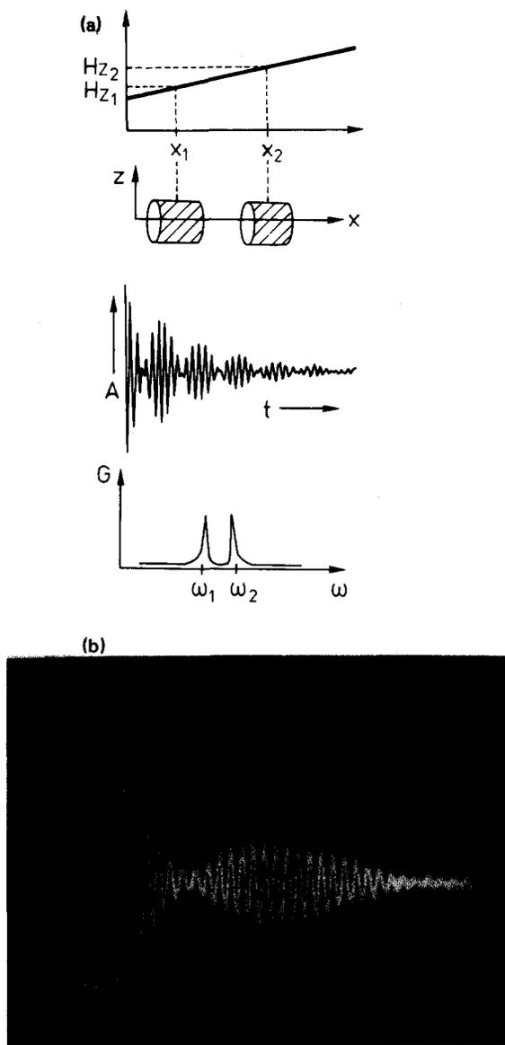
Fig. 6. (a) Signal form and frequency spectrum of a one-dimensional structure subject to a field gradient. Field gradient in  $x$  direction. Time and frequency domains are related by Fourier transformations. (b) FID of two  $0.1\text{-cm}^3$  glycerol samples spaced  $0.5\text{ cm}$  apart in a slightly inhomogeneous region of the field. The signals were averaged over 100 transitions using a Tektronix 7854 oscilloscope.
