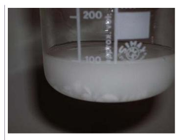
When two solutions were cooled, start to pour NaOH solution. Pour in the small amount, because all mix in the erlenmeyer flask will start to heat. So add it slowly and good stir after addition. Need to do this while you will see 2 layers and the ph will be 10-12. When the NaOH is added, wait while all
