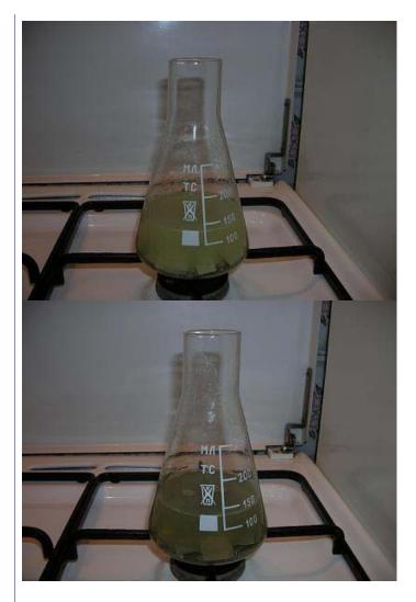
In this time, all solution will boil, so need to put in the erlenmeyer flask some condenser.
