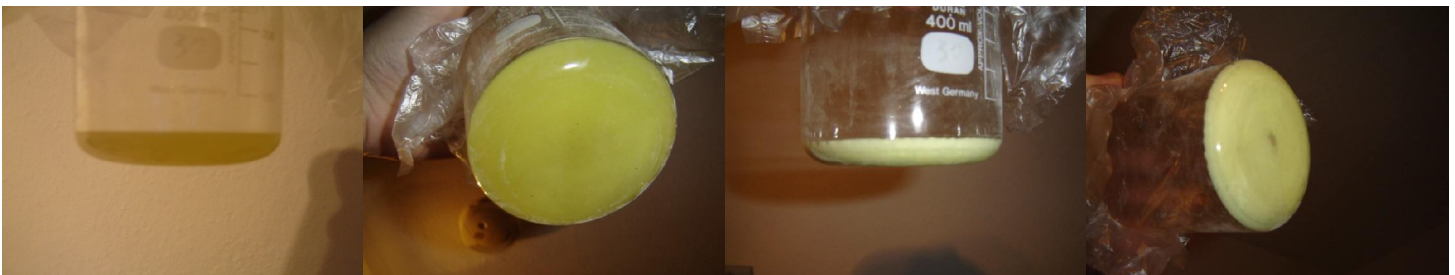
Here you can see the crystals forming while cooling down, in the buchner filter the crystals were washed with water.
