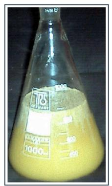
The oil was dissolved under stirring in 300mL GAA, and the flask placed in an ice-H<sub>2</sub>O bath. A solution of 53.3mL [166.2g; 1.04mol] Br<sub>2</sub> in 300mL GAA was added under stirring in one portion, and a reflux column was quickly attached. After ~1min the flask was removed from the ice-H2O bath and the rxn mixture left to stir at room temp. The flask became warm, and after approx. 6min spontaneously crystallised to a pale yelloworange unstirrable mass [Fig. 2 (left)].
