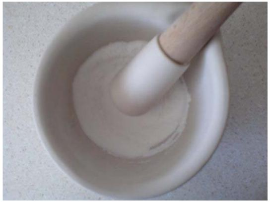
The tablets in the morter. They have to be grinded as fine as possible so the powder has the largest surface as possible. This improves the extraction.
