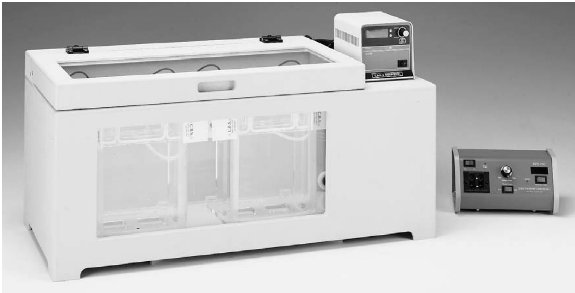
Figure 5 The entire automatic TDGS system. In this version of the system, four gels can be run simultaneously submerged in a buffer tank, which is equipped with a heater/stirrer to provide for a constant temperature. For more information, see http://www.cbssci.com
