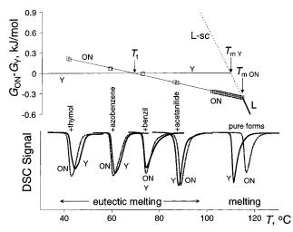
**Figure 5.** Illustration of the use of melting and eutectic data for determining the stability relationship between polymorphs. Bottom: melting endotherms of Y and ON as pure crystals and in the eutectics with acetanilide, benzil, azobenzene, and thymol. Top: the  $\Delta G - T$  curve calculated using eqs 1–3. The free energy of ON is plotted against that of Y (horizontal line). The ON and Y lines terminate at the liquid line (L: stable liquid, L-sc: supercooled liquid).
