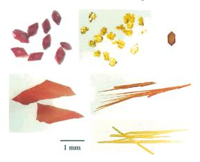
**Figure 2.** Photomicrographs of the polymorphs of **1**, showing different habits and colors. From upper left, clockwise: R, Y, OP, ON, YN, ORP.
