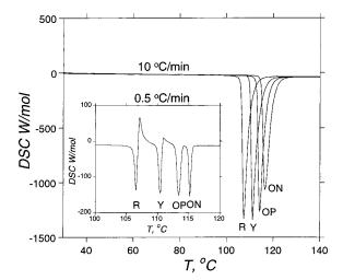
**Figure 3.** Melting endotherms of Forms R, Y, OP, and ON (left to right) recorded at 10 °C/min, each showing the homogeneous melting of a unique polymorph. Inset: DSC trace recorded at 0.5 °C/min of a polymorphic mixture, showing better separated melting endotherms and exotherms caused by crystallization from supercooled melt.
