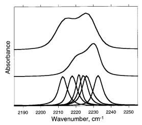
**Figure 7.** The CN stretch bands of **1**. Bottom (left to right): Forms R, ORP, YN, ON, OP, and Y. Middle:  $CCl_4$  solution (0.90 mM). Top: supercooled melt at 22 °C.
