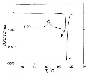
**Figure 4.** DSC trace of a sample of YN showing an exothermic conversion (Event C) and subsequent melting as R (trace amount) and Y. The area of C gives an estimate of the enthalpy difference of YN and Y. This experiment used a faster-than-normal heating rate (20  $^{\circ}$ C/min) in an (unsuccessful) attempt to observe the pure melting of YN. The faster rate caused thermal events to be more intense than those seen in Figure 3.
