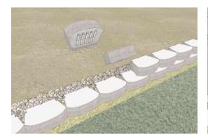
**Step 3 - Add More Courses** When building successive courses, center the first block on the two blocks directly below it. Using crushed drainage rock, backfill 12" behind each
