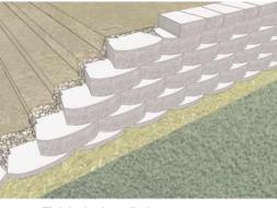
**Step 4 - Finish the Installation** Position the Mini Caps and adhere in place with Super-Stik<sup>™</sup>.
