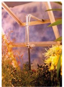
Solar-powered vent controls help automate the vetilation system.
