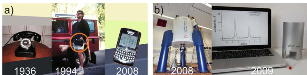
**Fig. 1.** Examples of miniaturization. Progressing miniaturization goes along with increased functionality. (a) Telephones. (b) NMR magnets for high-field NMR (left) and low-field NMR (right). The spectrum on the screen is from toluene in a 2 mm diameter sample tube acquired at 30 MHz with the magnet shown on the right [3,4].
