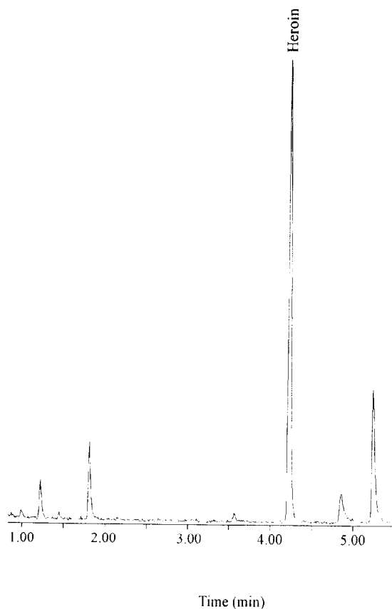
Fig. 5. Total ion chromatogram of the reaction product obtained from the reaction of 2 mg of heroin hydrochloride with 2 ml of acetyl chloride.
