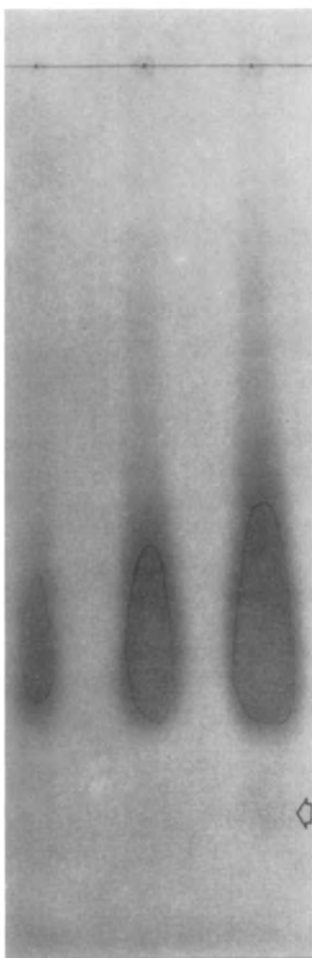
FIG. 2. Chromatogram of 25, 50, and 125 \mu\text{g} quantities of I developed in solvent system B and then sprayed with Schiff's reagent. A faint spot marked by the arrow is visible migrating ahead of the 125 \mu\text{g} quantity of I. The faint darkening along the solvent front is due to Schiff-positive material of the chromatography paper (see legend for lower plate of Fig. 1).
