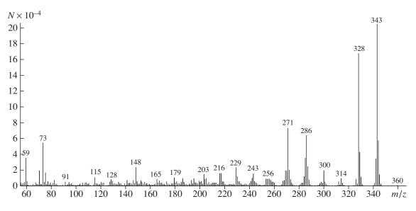
Fig. 4. Mass spectrum of the trimethylsilyl derivative of desomorphine (retention time, 18.897 min).
