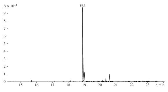
Fig. 3. Chromatogram of the trimethylsilyl derivative of desomorphine.
