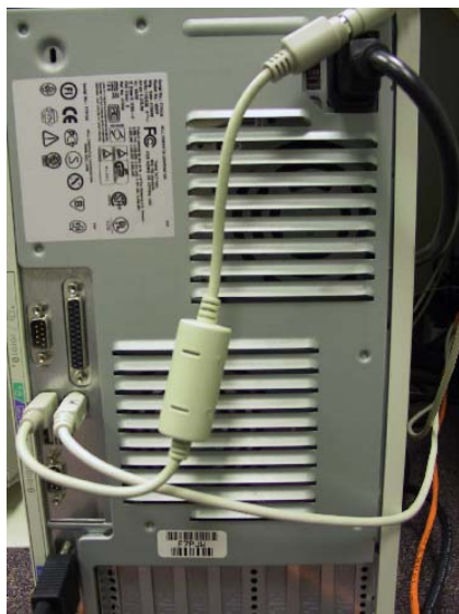
Keyboard cable with KeyGhost installed
