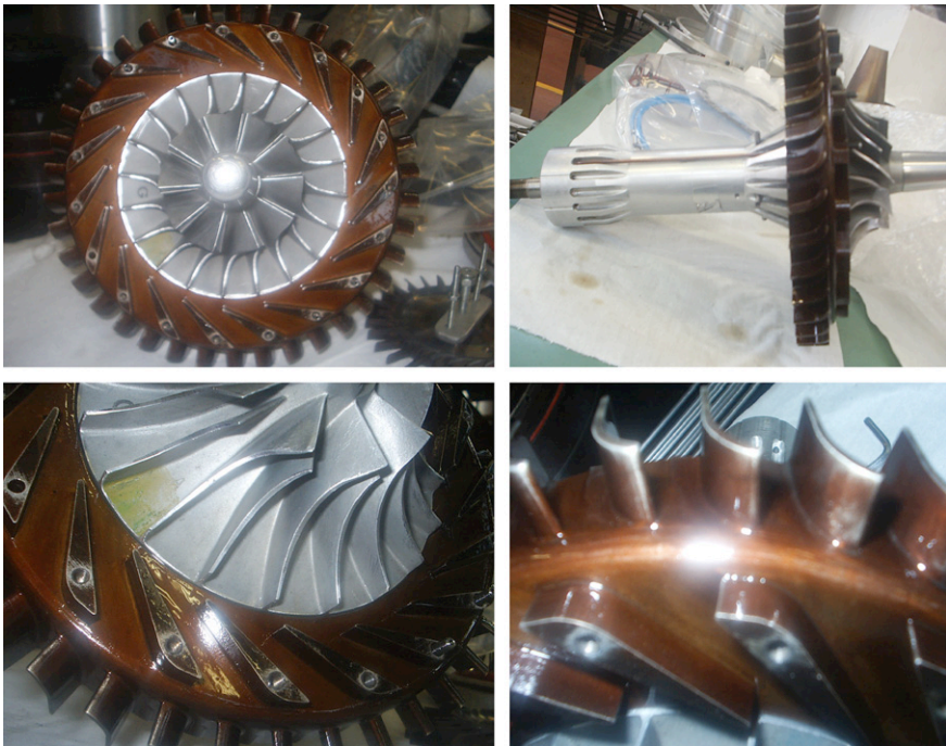
Fig. 3. Photos of the manufactured compressor.
