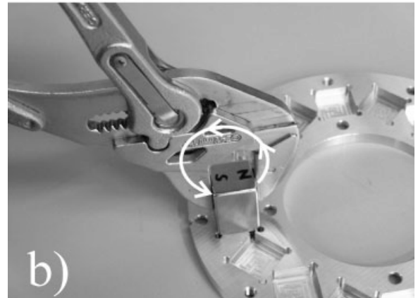
Figure 6 (a) Support ring showing the 16 5.7-mm deep sockets for the magnets. They were milled out from 6-mm sheet aluminium. The depths of the sockets were 5.7 mm. The “spiral” structure on the bottom of each socket is merely the path of the milling tool. (b) Magnetic “shorting” of a magnet by the use of a pair of ferromagnetic pliers.
