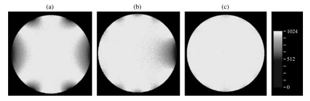
**Fig. 4.** NMR tomograms of a cylindrical sample of water (layer thickness, 5 mm), obtained by using (a) saddle coil; (b) birdcage resonator; and (c) our coil. A signal-level gradation scale (in conventional units) is shown at the right of the figure.
