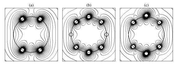
Fig. 3. Contour diagrams of the magnetic field in the coil midsection: (a) saddle coil; (b) birdcage resonator; and (c) our coil. The lines are drawn with a step of 0.05; the field at the center is assumed to be 1.
