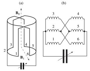
**Fig. 2.** (a) 3D presentation and (b) circuit diagram of an NMR probe coil.
