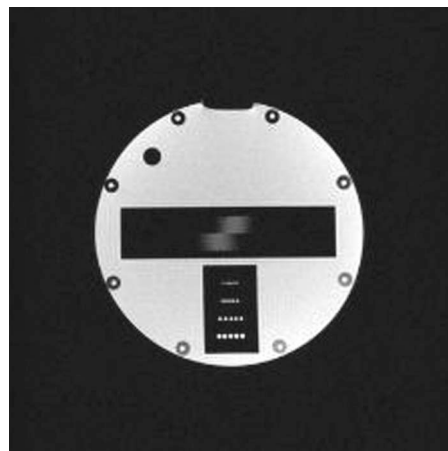
FIG. 8. T1-weighted image of a round phantom (140 mm diameter) obtained with spin echo pulse sequence in a 0.5 T permanent magnetic system. The experiment parameters are as follows: SF=21.3 MHz, P90 = 3.072 ms, TR=460 ms, TE=18 ms, number of excitations NEX=2, acquisition matrix size is 256 \times 256, field of view FOV=250 \times 250 mm 2 , slice thickness=7 mm, signal sampling rate is 50 MHz, and receiving bandwidth is 50 KHz.
