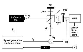
Fig. 1. Setup of the velocity servo control loop of the target mirror. SM: Stationary mirror, MM: movable mirror, PBS: polarization beamsplitter, QWP: quater wave plate, HPTS: high precision translation stage, PZT: piezoelectric actuator, Int: integrator, MP: mixing polarizer, DDS: digital direct signal generator. The signal generator is controlled by a computer (PC) via an IEEE communication port.
