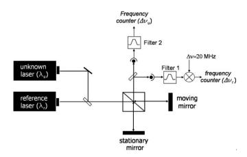
Fig. 3. Experimental setup of the wavemeter. Two frequency counters measure the Doppler frequency shifts due to the moving mirror for both lasers. The filter 1 is a band-pass filter centered around 20 MHz. The filter 2 is a low-pass filter (cut-off frequency = 30 kHz). As the reference laser has two optical components separated in frequency by 20 MHz, it is first demodulated before reaching the frequency counter. The unknown wavelength is determined thanks to Eq. (3).
