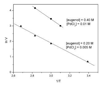
**Figure 1.** Palladium-catalyzed oxidation of eugenol: temperature effect. *Conditions:* gas phase  $O_2$ , 10 atm; solvent DMA/H<sub>2</sub>O (20 vol%).
