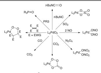
**Fig. 4** Known reactions of  $(L_n)Pd(\eta^2-O_2)$  complexes
