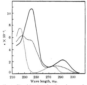
Fig. 1.—Ultraviolet absorption of tyrosine at various pH values: ...., pH < 8; ---, pH = 10; ---, pH > 12;  $\epsilon = D/cl, c = \text{concn. in moles/l.}, l = \text{path length}, D = \text{optical density as read by Beckman spectrophotometer.}$
