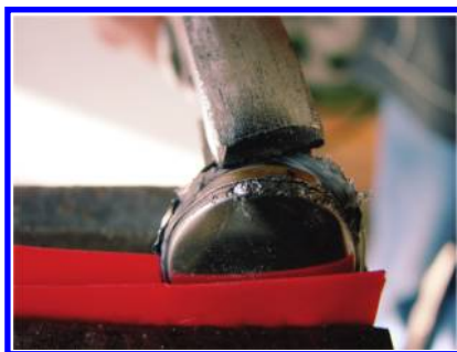
Figure 2. Opening a Li battery. Some form of insulation is advisable to prevent the battery from discharging by short circuit with the vise's metal.
