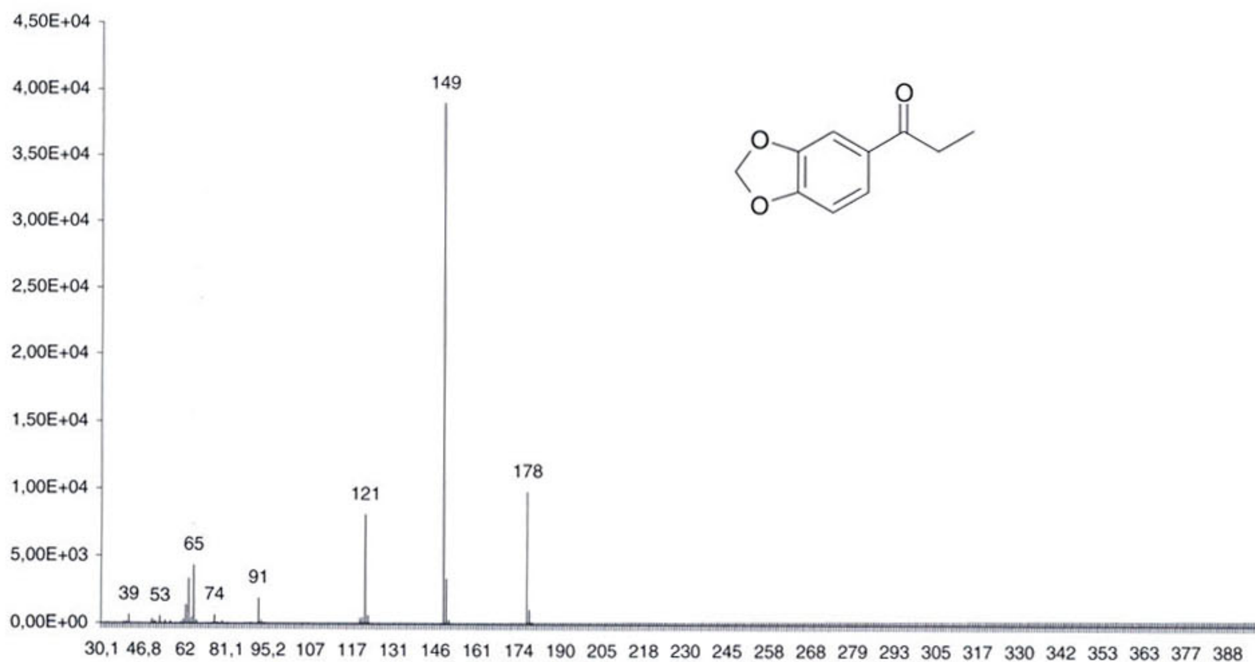
Fig. 6. Mass spectrum of 1-(3,4-methylenedioxyphenyl)-1-propanone (compound 10 in Table 2).
