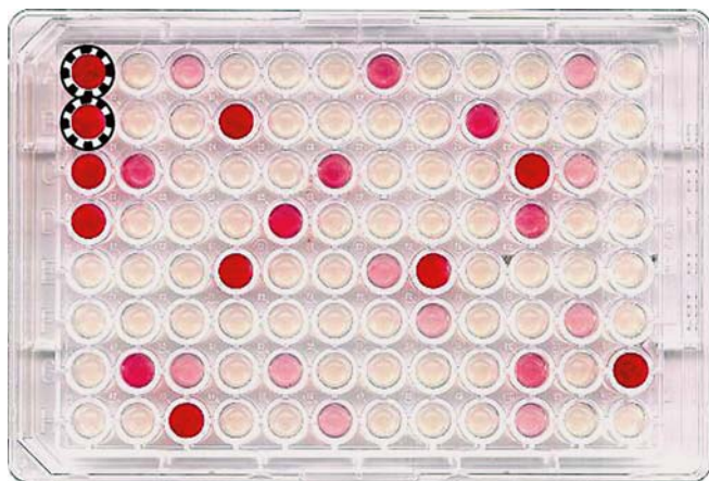
Fig. 5 Microplate with different variants of pyruvate decarboxylase. Cells were lysed and incubated for ( R )-PAC synthesis. ( R )-PAC was detected by use of tetrazolium red as described above. Standard clones are highlighted
