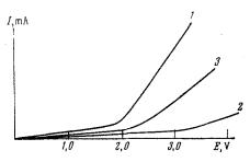
Fig. 1. Anodic oxidation of benzene on Pt in acetonitrile on a  $(C_2H_5)_4NF \cdot 3HF$  support: 1) solution of  $(C_2H_5)_4NF \cdot 3HF$  before electrolysis; 2) after preliminary electrolysis at 2.9 V (s.c.e.); 3) solution of 1.0 g of benzene and 5.0 g of  $(C_2H_5)_4NF \cdot 3HF$  in 30 ml of acetonitrile after preliminary anodic polarization.
