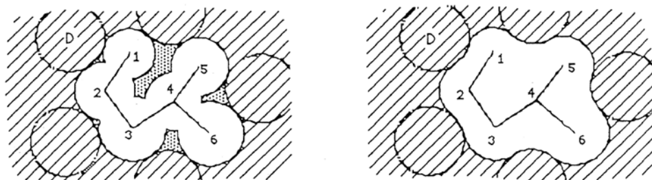
Figure 2.1.7. The Solvent Excluding Surface of a particular solute is the envelope of the volume excluded to the solvent considered as a whole sphere that represents its charge density.
